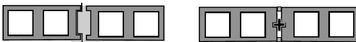
Figure 1: Shrinkage Control Joints (From Klingner 2010)
