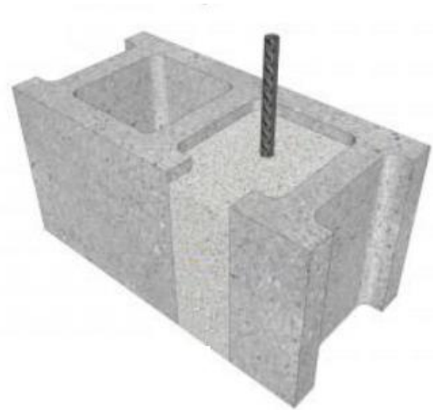
Figure 5: Faceshell removed to install rebar and grout
