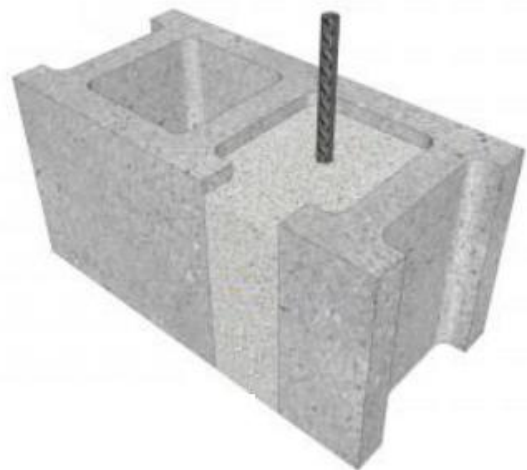
Figure 2: Sawcut vertical rebar in existing masonry core from IMI Masonry Detail Series http://imiweb.org/masonry-detailing-series/
